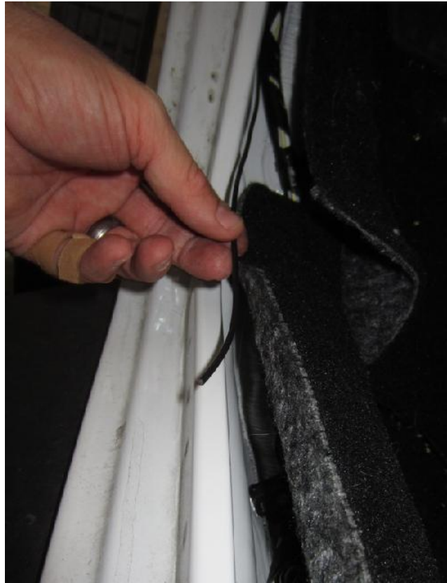
Figure 1: Black Wire run down sill
